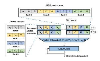
Figure 3: Exploiting inter-bank parallelism in dot product computation of one BBS matrix row and the dense vector.
