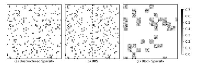
Figure 2: Weight map visualization after pruning with (a) unstructured sparsity, (b) BBS, and (c) block sparsity (sparsity ratio = 90%). These weight maps are  $64 \times 64$  sub-matrices of the whole  $1500 \times 1500$  matrix.
